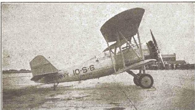
This trim craft is the Navy Vought "Corsair" O2U-4 which is used by the Navy Scouting Squadrons and thrown from cruiser catapults. A single-seater of fine performance, it carries much Navy equipment, such as deck-landing gear and flotation bags.
